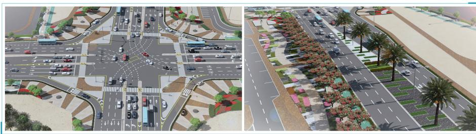
Tatweer has successfully completed the design of the signalized intersection upgrade of Al Ain Hospital in Al Ain City. The executed scope included roadway geometry, traffic system, landscape, street lighting and storm drainage design. The project objective is to improve the traffic flow for both drivers, pedestrians, and the ease of access to Al Ain Hospital and the governmental offices around the Baladiyah Park.
