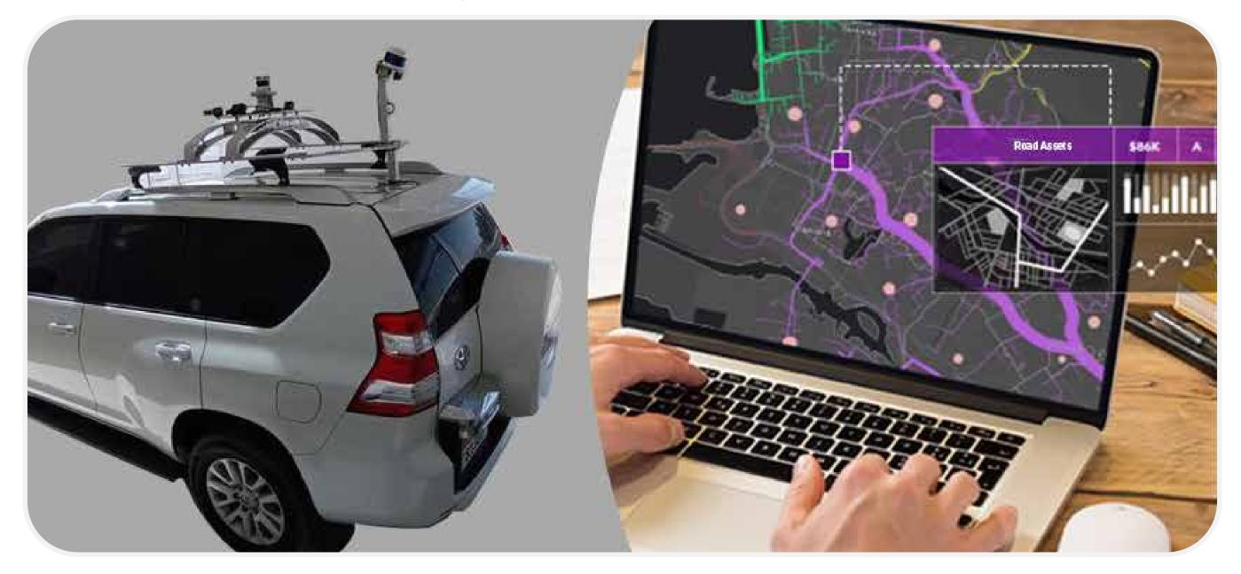
As a continues improvement for road infrastructure operation and road safety, our R&D team started development of new product "**Intelligent City Mapper**" using AI, remote sensing, 3d mapping and geospatial technologies to collect all road data objects such as signboards, distortions, pavement, road furniture's with accurate locations on one collaborative platform and visualize the outputs on an informative GIS based dashboards.
